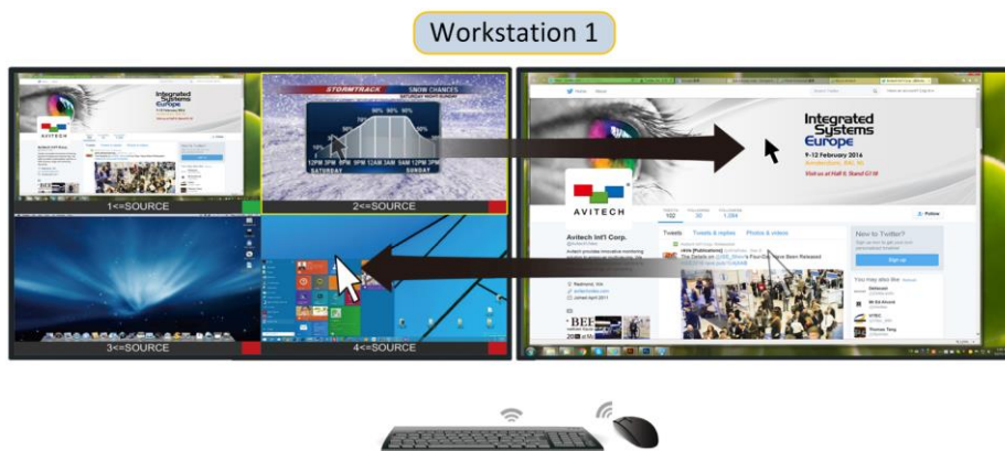
Figure 3.3.1.4 “Surfer” Feature on Two Display Monitors
